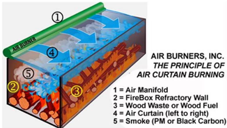
A secondary benefit is the great speed at which waste burns – often 10 times as fast as an open burn. Containing and extinguishing the fire, if necessary, are also fast and relatively easy. The benefits of such incinerators in the aftermath of a tornado or a hurricane are obvious.
