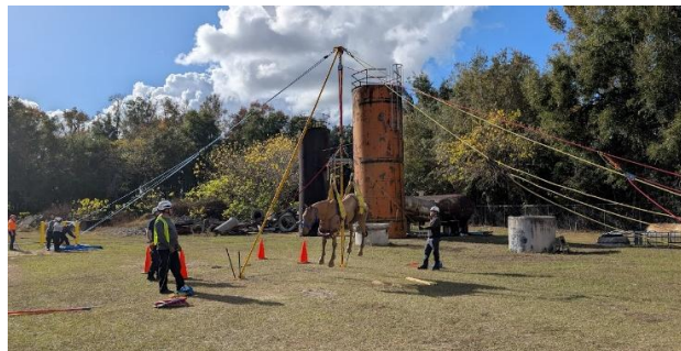
Right: Vertical lift of a large animal using a portable high point anchor system, December 2024
