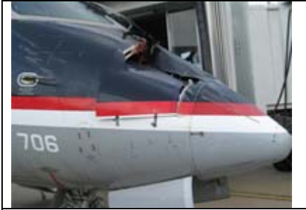
Damage to nose of jet airplane caused by bird strike. (USDA-APHIS photo)
